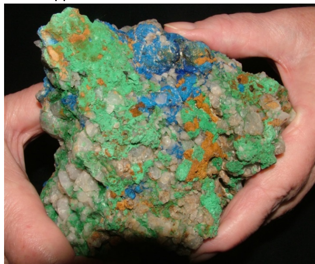
Figure 1 Example of Wheal Barton high grade copper carbonate mineralisation.
