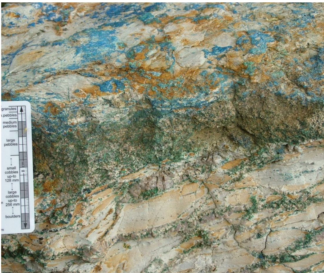
Figure 8 Quartz veining with copper carbonate in spoil at sample location 265568 (refer to Figure 1).
