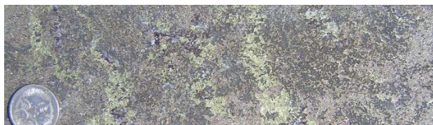
Figure 5: Sulphide-rich zone containing abundant sphalerite (black), chalcocopyrite (yellow), galena (blue grey) and pyrrhotite (bronze) at 204.25m in hole EL14D12.
