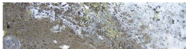
Figure 4: Compositionally banded sulphide-rich mineralisation containing pyrrhotite (bronze), chalcopyrite (yellow), sphalerite (black) and calcite (white to pale grey) at 198.45m in hole EL14D12.
