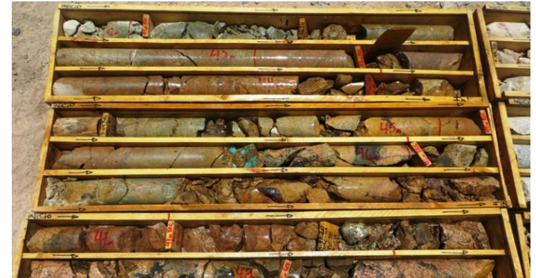
HQ diameter diamond core from hole DHC-01 at Colupo identifying copper mineralised breccia intercept at approximately 43 metres to 51 metres downhole (January 2014).
