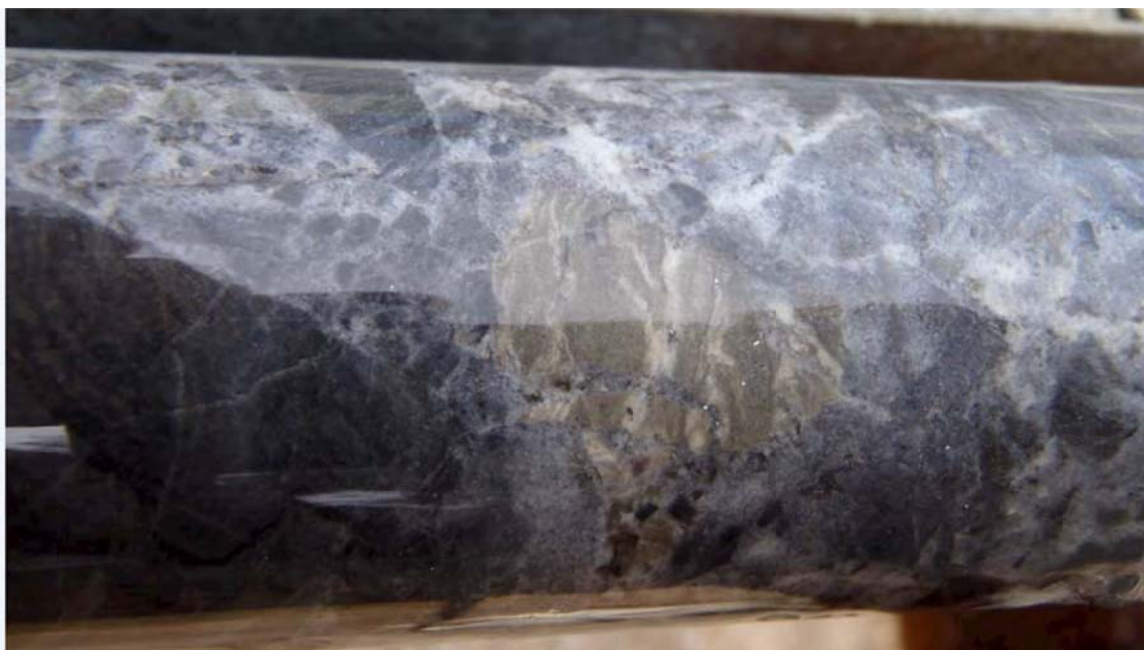
Core, SGRDD43. Brecciated metasediments exhibiting quartz-sulphide-felsic dyke flooding from 32.00-33.00 metres downhole (field of view L-R 70mm). The light brown material in center of the core is a finger of dyke with disseminated sulphides (BQ Core 36.40mm diameter).
