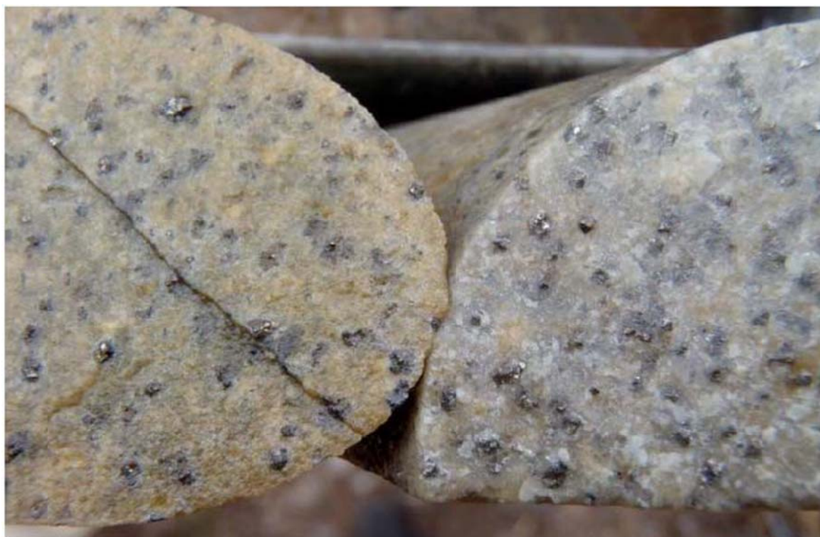
Comparison of core samples of altered felsic dyke in SGRDD0043 with SGRDD004 from Martins Shaft. This figure shows the surfaces of sheeted vein alteration in felsic dykes studded with 0.50-2.00mm wide sulphides (field of view L-R 65mm). SGRDD0043 (LHS, 23.40m downhole) and SGRDD004 from Martins Shaft (RHS, 47.45m downhole).
