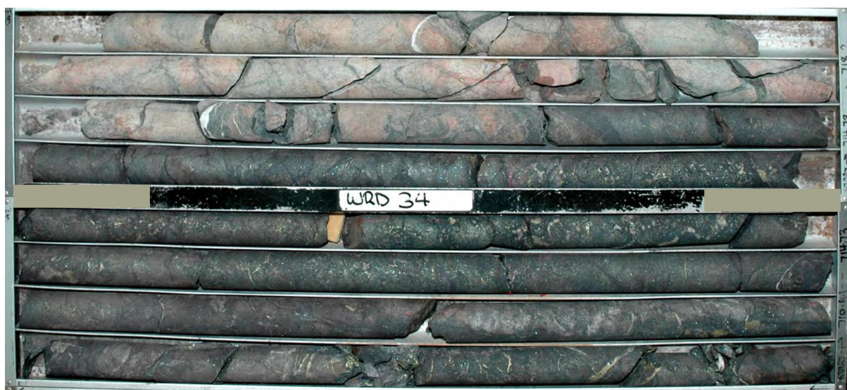
Figure 2 (BHP): Dry core photo (circa 715m) of weakly brecciated, iron oxide altered and mineralised mafic-ultramafic at Wirrda Well IOCG deposit located 20km south of Olympic Dam
