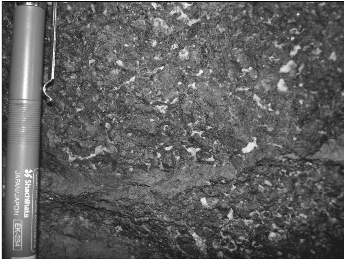
Figure 10. Handspecimen photo of Datong “Qijiang Style” mineralisation taken from a face of mineralisation underground. The photo shows brown, pale brown hematite/goethite/siderite and interstitial pale crème silica.
