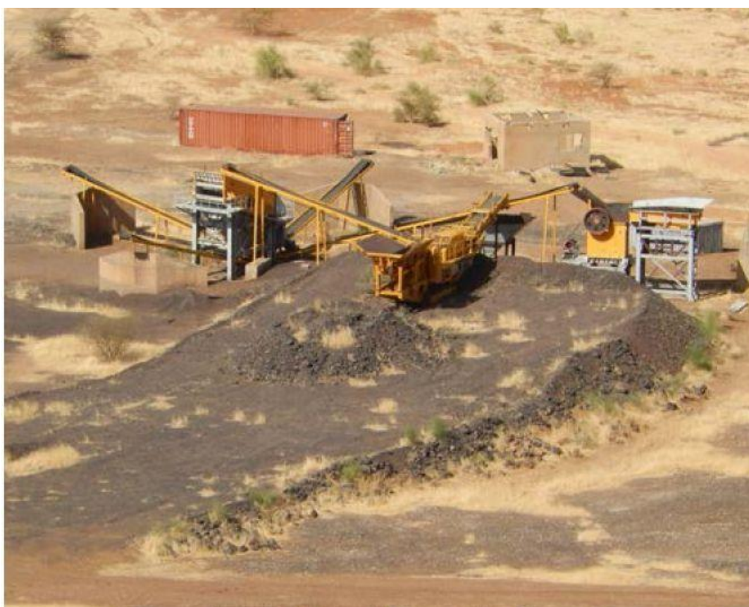
Figure 6: Crushing and screening facility at Takavasita (Coffey 2014)
