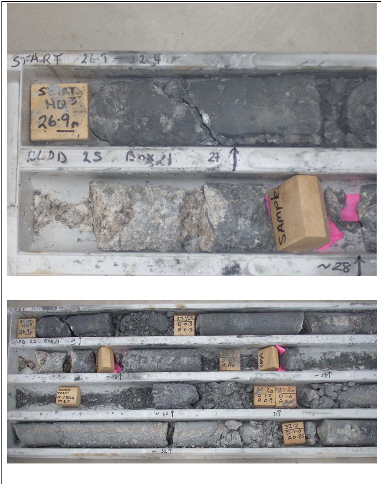
Figure 14. BLDD025: Top – high-grade oxide graphite at 26.9 m. Bottom – graphite beds from 26.9 m to 32.2 m; some removed for assay and metallurgical work (Sample). Note that from 30.2 m to 31.2 m there was zero recovery of a graphite bed.
