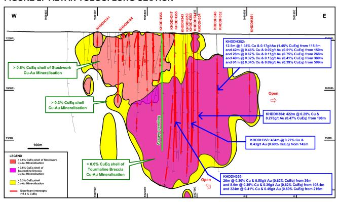
Altan Tolgoi long section showing recently completed drill holes.
