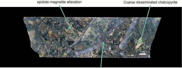
Sheeted quartz-chlacopyrite veins
