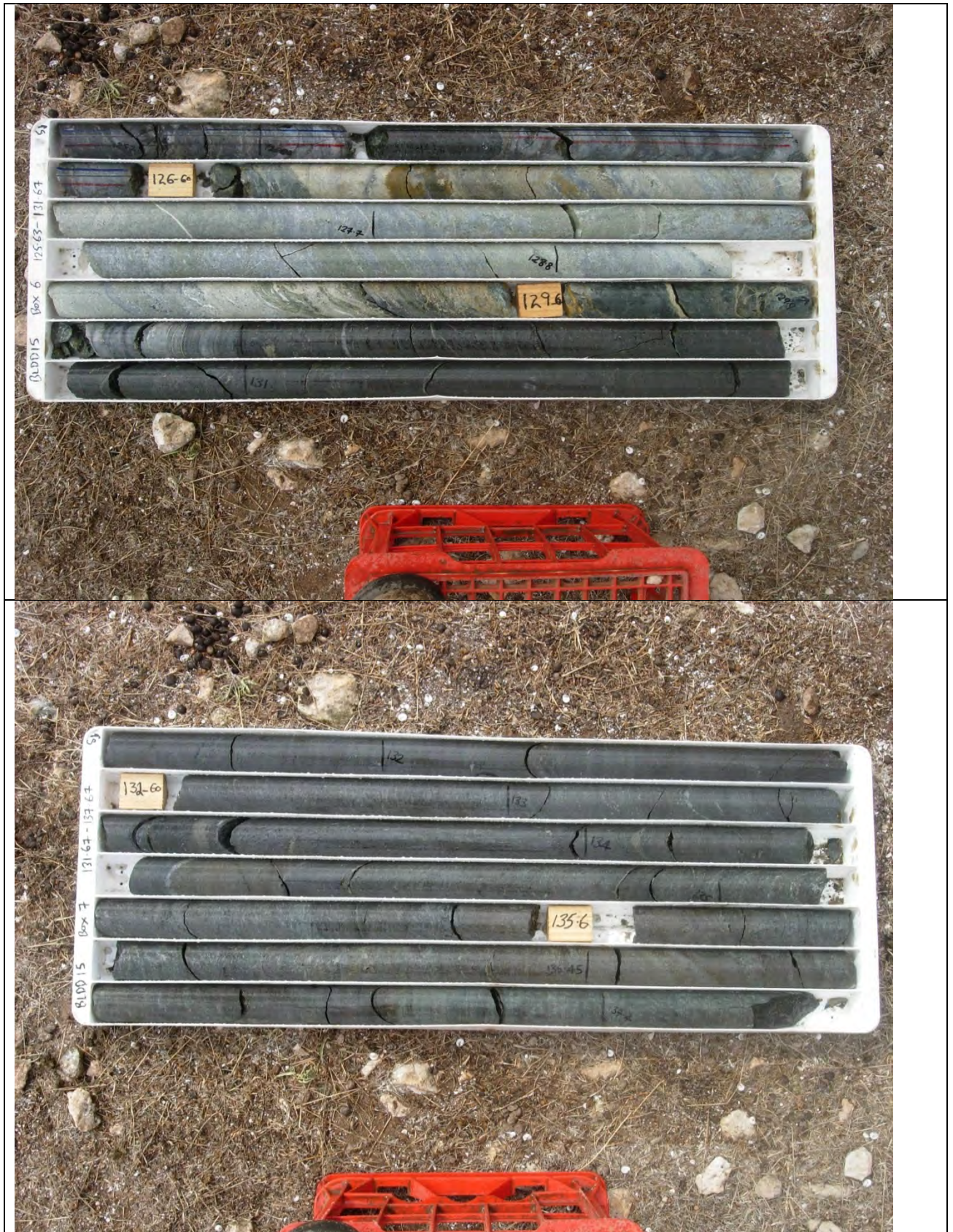
Figure 13. BLDD15 –Photograph of part of the primary graphite bearing units (from ~125 m to ~138 m)
