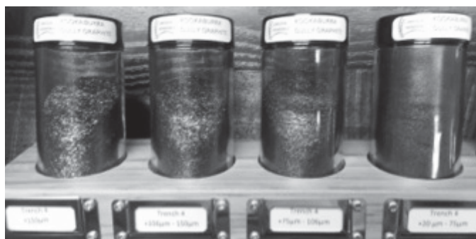
Laboratory-scale flotation tests on a Kookaburra Gully bulk trench sample and resultant graphite flake concentrates grading from medium-coarse flake (left) to fine flake (right)
