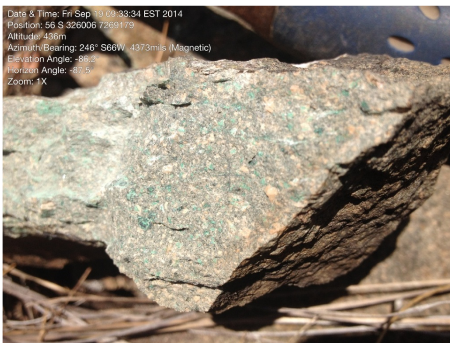
Figure 3. Copper bearing porphyritic dyke. Rock Chip 3011274 (0.87% Cu)
