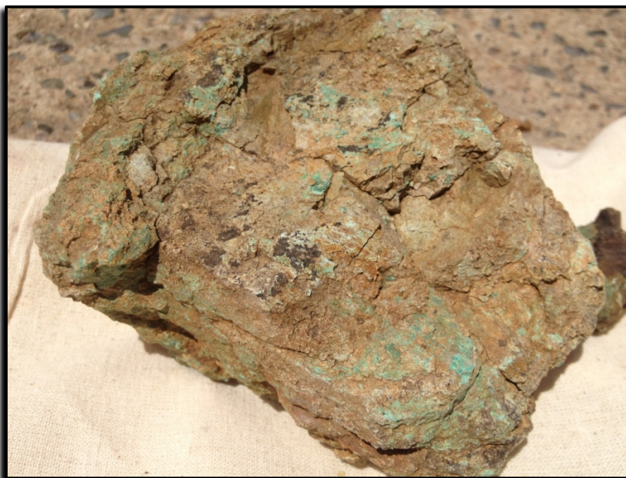
Figure 4. Strong Copper Oxides developed in brecciated sediments adjacent to porphyritic dyke. Sample 3011273 (24.2% Cu)
