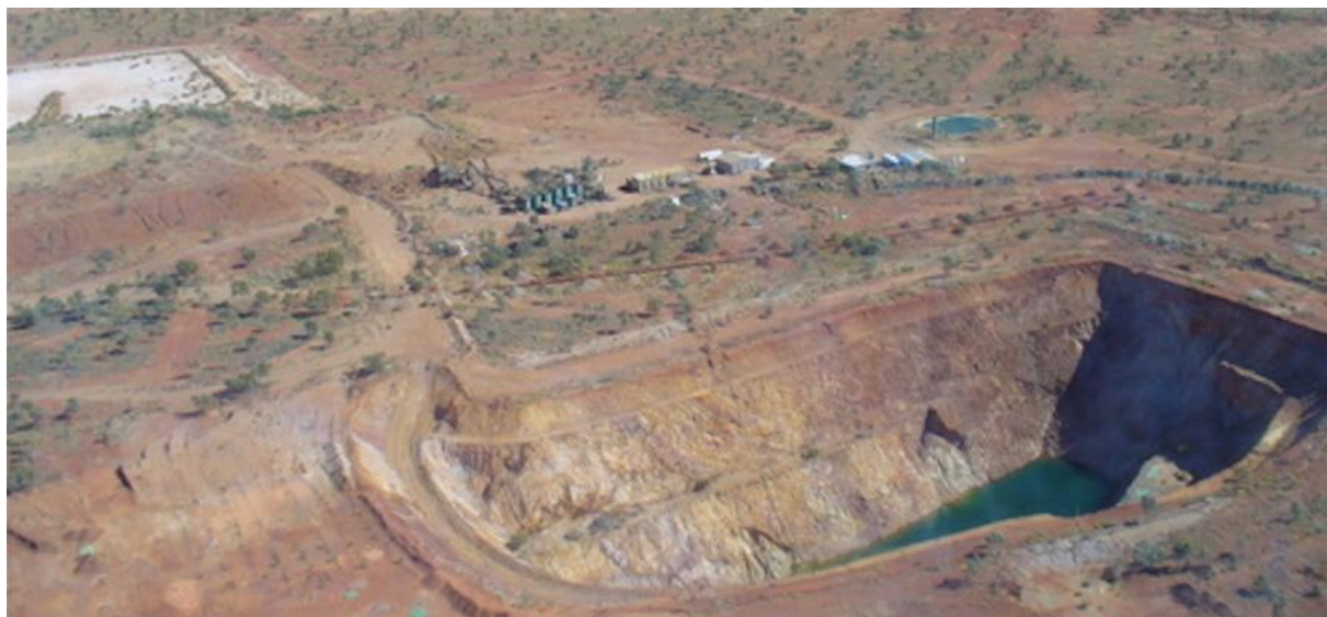
Nicolsons Mine, the focus of works at Halls Creek, with open pit in the foreground, processing plant and surface facilities centre, and existing tailings facility at top of picture.
