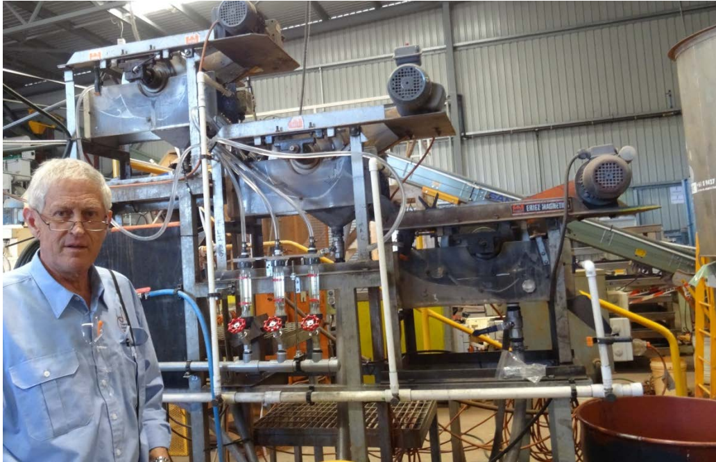
Technical Director Ray Koenig and the cleaner magnetic separator top, Hydroseparator column right
