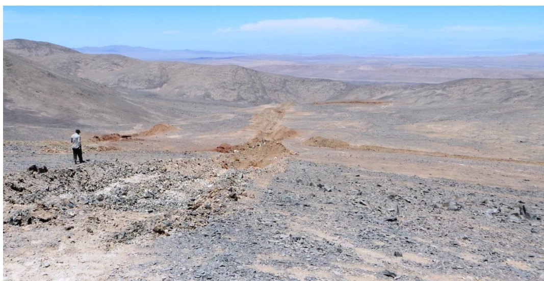
Figure 7: Trenches at Colupo Norte, dug historically by SQM, exposed copper oxide within breccia (view NE).
