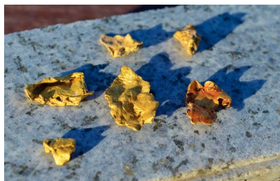
Photo of gold "flakes" found in the high grade target area after bulk sampling had taken place. The gold was found as free grains within the altered granite and clay surrounding numerous small quartz veins. The largest of the grains (in the center of the photo) is 22mm long and 12mm wide. The grains are photographed on a small slab of tonalite, the typical host rock of the area.
