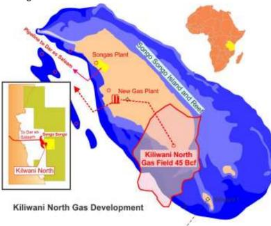
Kiliwani North 1 tested at 40 MMcfg/day from the Kiliwani North Pool located only 2 km. from the new Songo Songo gas plant and pipeline to Dar es Salaam.
