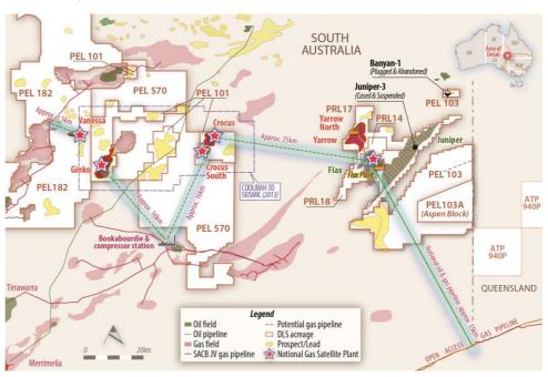
step out appraisal well and the first well drilled in the Juniper field using 3D seismic. The well is located approximately 6km to the northeast of the Juniper-1 discovery well and encountered pay intervals in the lower Patchawarra Formation. The well successfully established the northeast extension of the field and was cased and suspended for future testing and hydraulic stimulation.
