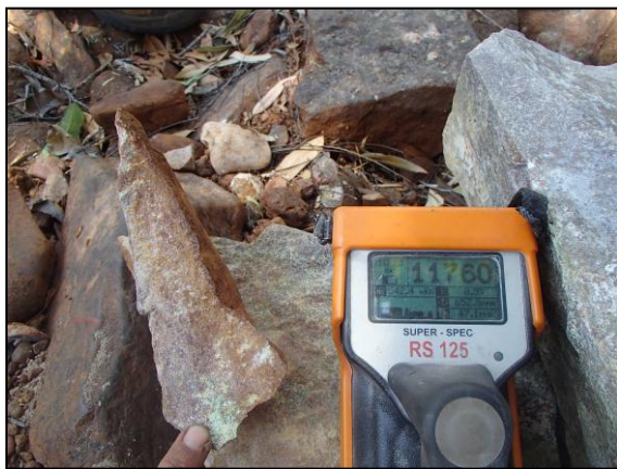
Figure 2. Photos of strong visible primary and secondary uranium mineralisation identified in Steptoe fault zone.
