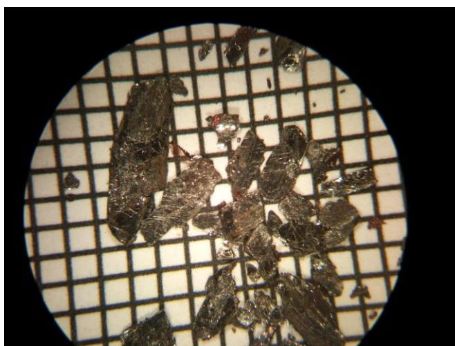
Plate 5. Argent graphite prospect ultra-coarse graphite released by knapping a surface rock. Note: the square scale grid is 1 millimetre
