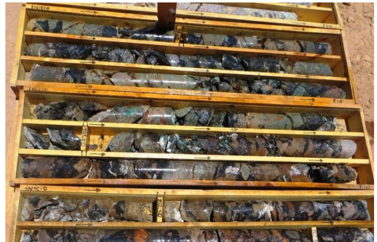
HQ diameter diamond core from DHC-02 at Colupo identifying intercept 97 metres to 104 metres with visual extensive tourmaline filled breccia with copper mineralisation (January 2014).
