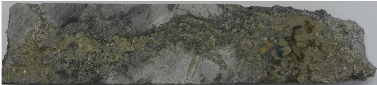
Figure 4 Chalcopyrite (pale yellow) and pyrite (yellow) veins in silicified and carbonate altered black slate host (width of core photo is 45mm)
