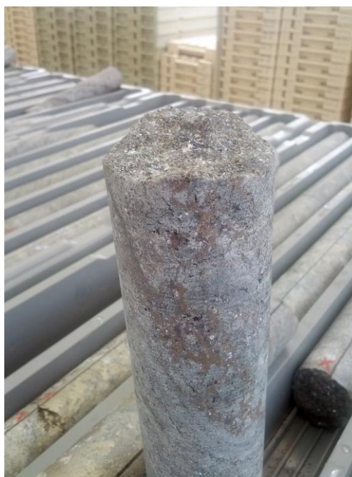
[Figure 1] Maronan Project: MRN14007 coarse grain size, remobilised lead mineralisation typical of the higher grade "Bonanza" style from the apex of the northern fold structure.
