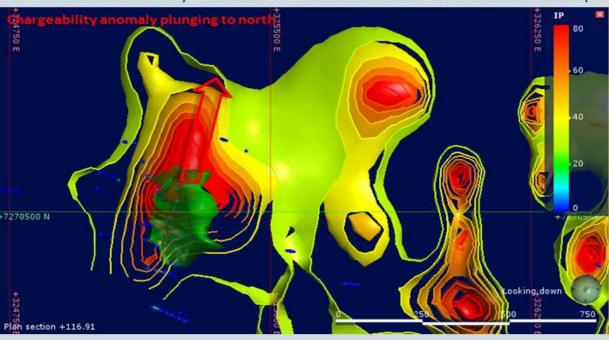
. Plan View – Elevation slice 120mRL illustrating zone of high chargeability (yellow-red) adjacent to and to the north of the current Mt Cannnindah Cu-Au Resource (green)
