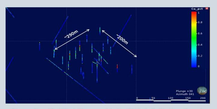
Oblique 3D Long section of the United Allies prospect looking NE, illustrating the dimensions of mineralisation and lack of drill testing at depth.
