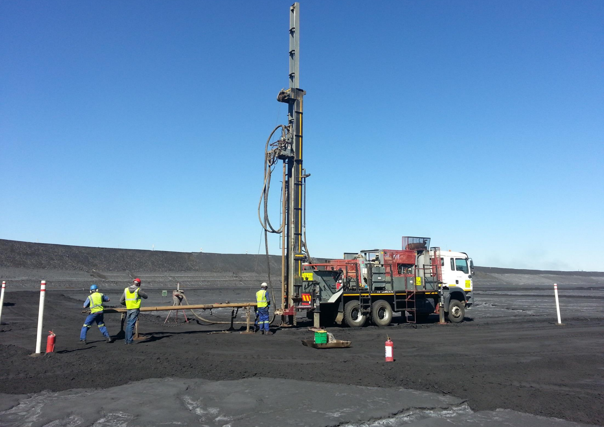
Anglo American representatives conducting coal fines sampling as part of the Detailed Feasibility Study with RESA
