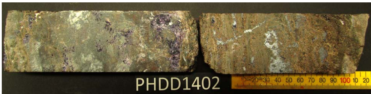
Plate 1. Drill core from 922.45m - 922.75m showing zone of chalcocite (steely grey colour) and fluorite (purple colour) mineralisation. 1m zone 922m - 923m assayed 1.4% Cu, 0.12 g/t Au and 36g/t Ag (downhole length reported).
