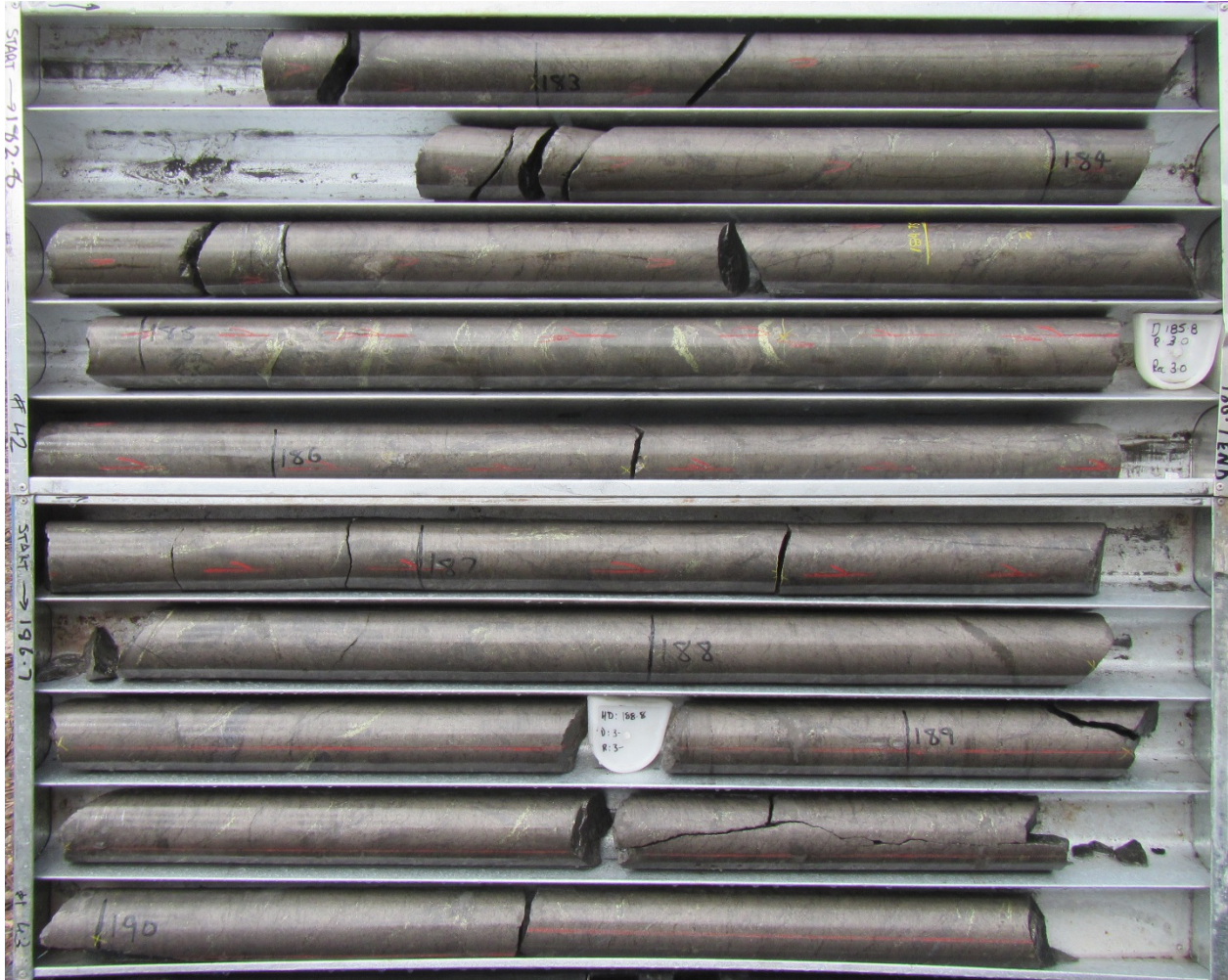
Figure 1: Iron Blow drill hole IBDH23 showing interval of massive sulphides from 182.8m (top left) to 190.7m (bottom right). This is from an interval of massive sulphides from 156.5m to 206.1m downhole. The brassy coloured sulphides are massive pyrrhotite with darker zinc sulphide (sphalerite). Bands of yellow chalcopyrite are clearly visible.
