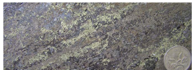
Figure 4: Compositionally banded sulphide-rich zone at 164.1m in hole EL14D21 containing sphalerite (dark grey), chalcocopyrite (yellow), pyrrhotite (bronze) and calcite (light grey). Part of a 1-metre interval assaying 3.9% Cu, 3.6 g/tAu, 14.6% Zn and 146 g/t Ag.
