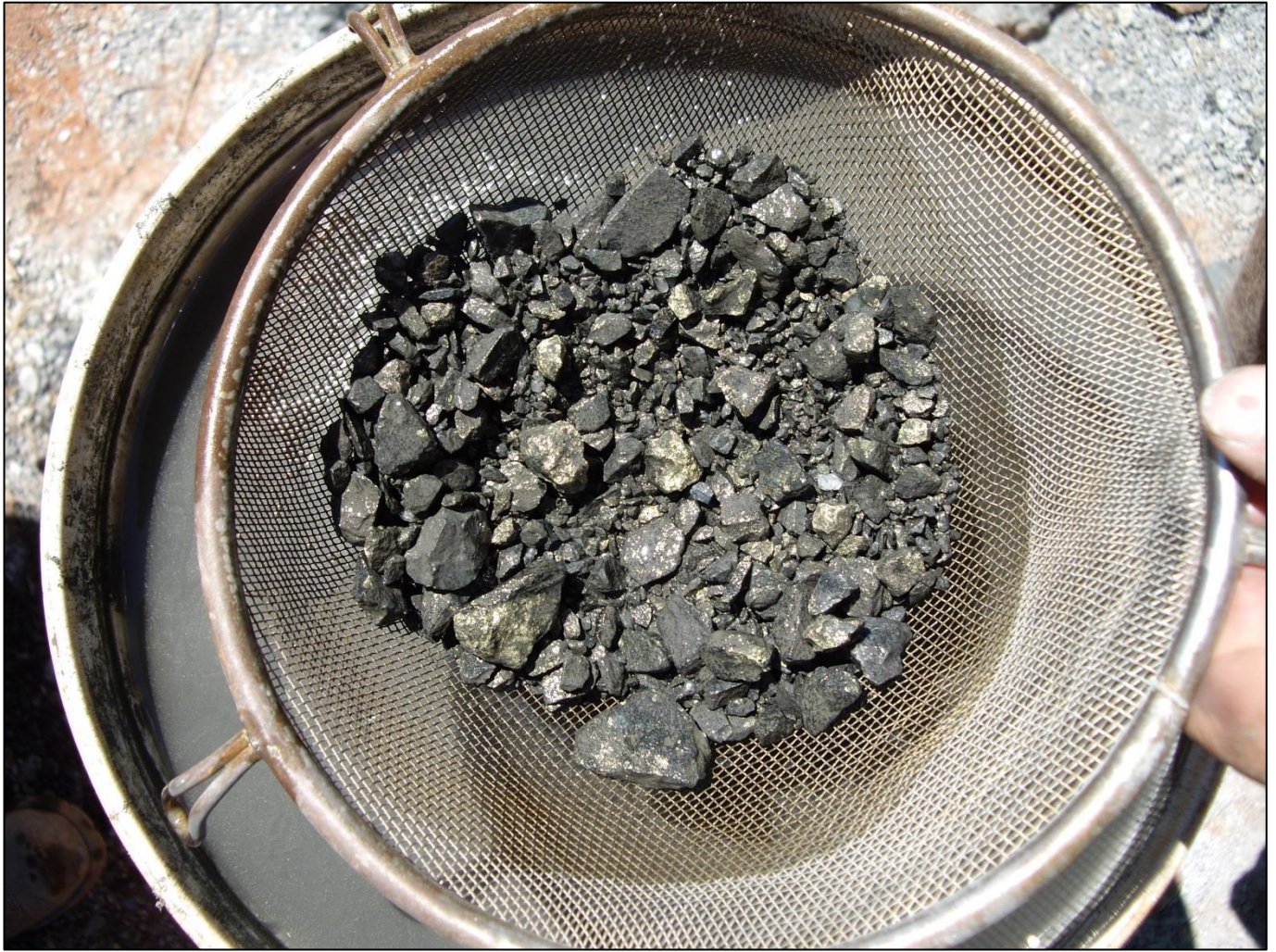
Figure 3: Sieved RC drill sample from NRC14008 – 197 to 198 metres showing abundant chalcopyrite (yellow)
