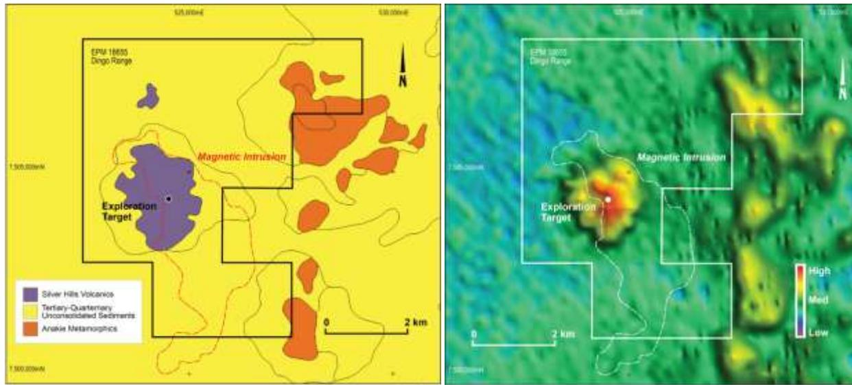
Figure 7. EPM 18655 Dingo Range showing exploration target area over interpreted geology (left) and radiometric imagery (right)
