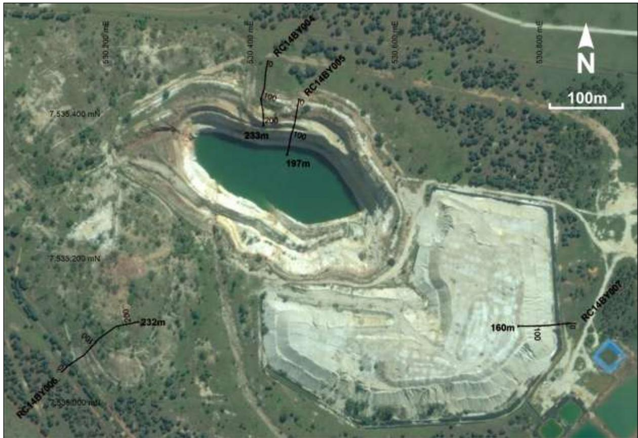
Figure 3. Location of RC holes on aerial photo image of the Belyando open-cut
