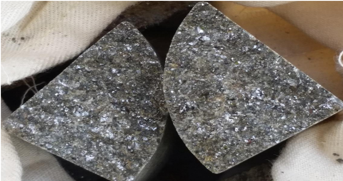
Figure 4: Cross-section of as-received quarter core from Block F South with visible graphite flakes
