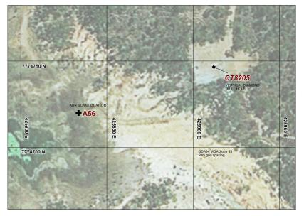
Map showing the location of ADR scan A56 relative to vertical diamond drill hole CT8205. The drill hole and scan was carried out in the "Imperial" area and targeted the E07 structure. Drill hole is a vertical drill hole with a maximum depth of 537metres. *Grid is MGA94 Zone55, 50m spacing*
