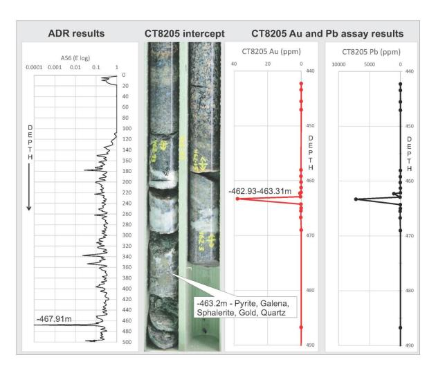
Above is composite diagram showing ADR geophysical scan results with a pronounced anomaly at -467.91 meters. The intercept in parallel diamond drill hole CT8205 is also shown along with assay results for the intercept. The intercept contained 37.9 grams per tonne gold and 7200 ppm lead at a depth of approximately -463.2 meters depth. Note the depth scale on the ADR scan and the drill hole assay results.
