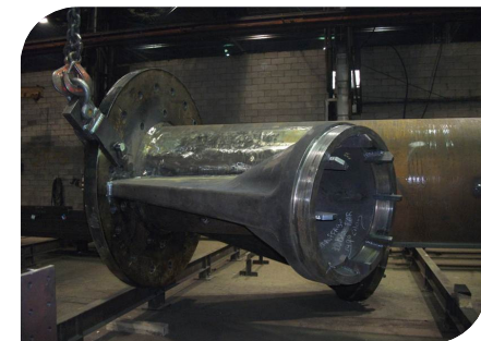
Arthur Ashe Tennis Stadium Node for roof support - Structural
