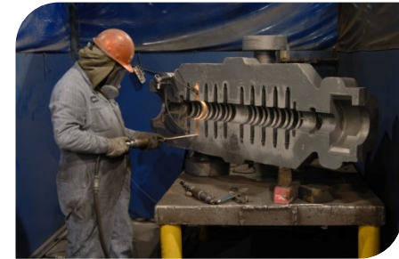
Multi-Stage Pump Casting with intricate clean passage requirements - Energy
