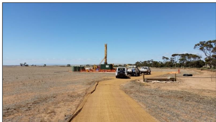
Photo 1: Northern Yorke Peninsula - Utilising environmentally sensitive techniques to minimise disturbance to the farmland, including the laying of 'coconut fibre matting' for all vehicles to drive and park on at the drill site
