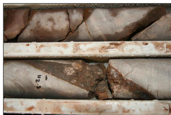
Photo 3: Spyall core at 112m - showing a haematite vein in basement metasediments
