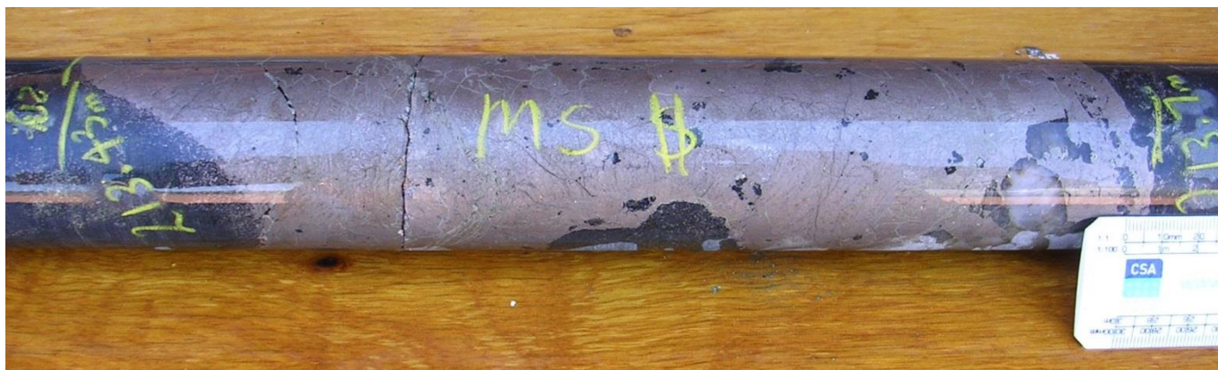
Figure 4: Massive sulphides (pyrrhotite and pentlandite) at 213.43m downhole in NRD15001. Length of NQ core in photo approximately 0.4 metres
