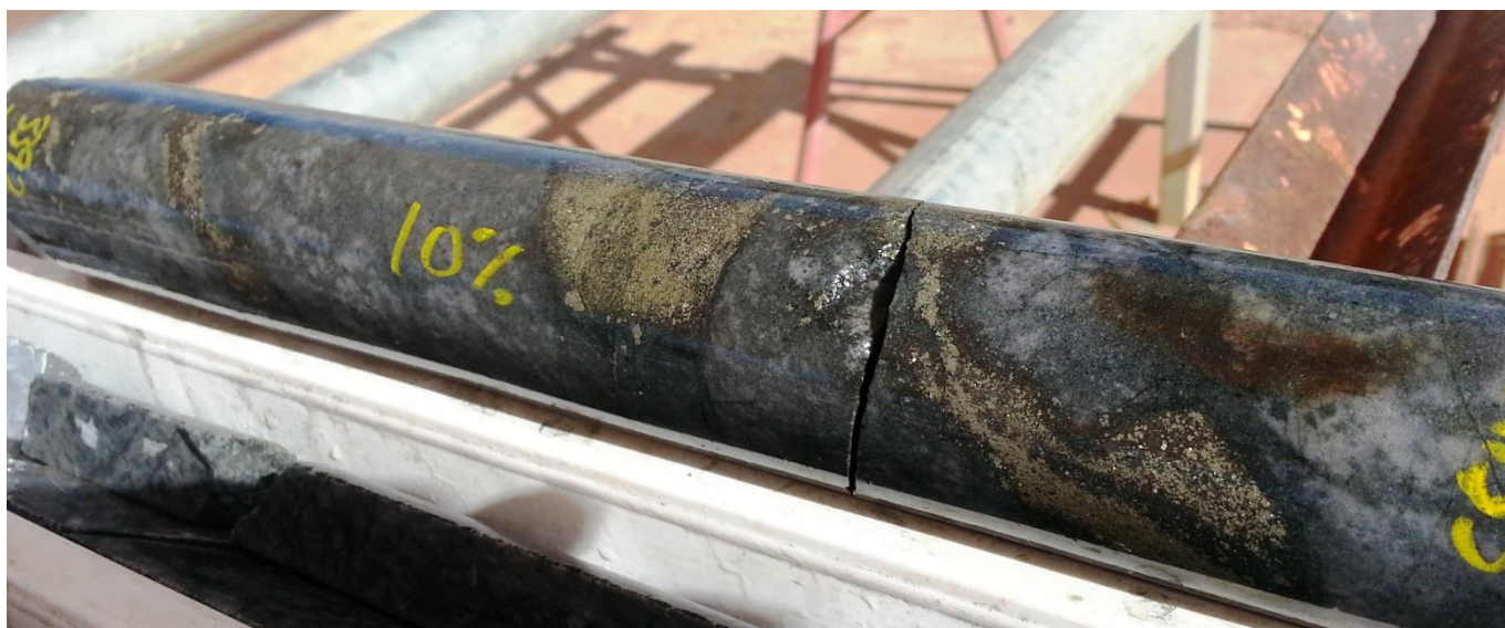
Figure 7: Stringer sulphides (chalcopyrite and pyrite) at 340m downhole in NRD15002. Length of NQ core in photo approximately 0.7 metres.
