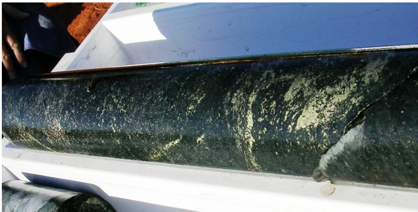
Figure 5: Disseminated sulphides (chalcopyrite) at 213.8m downhole in NRD15001. Length of NQ core in photo approximately 0.5 metres
