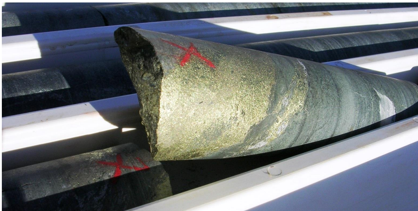
Figure 6: Massive / stringer sulphides (chalcopyrite) at 246.35m downhole in NRD15001. Length of NQ core in photo approximately 0.2 metres.
