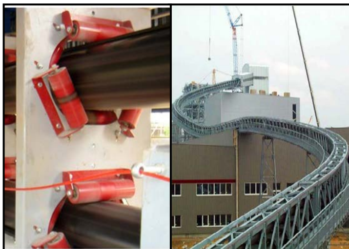
Figure 2 Pipe conveyor system at Port Pirie
