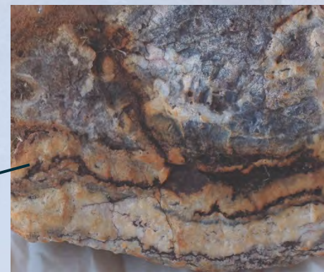
Colloform banded vein assaying 2.75g/t Au (gold zone texture)
