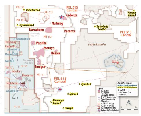
The fifth well in the current eight-well campaign, Kyanite-1, spudded on 23 February 2015 in PEL 513. Kyanite-1 is a near-field exploration well targeting the hydrocarbon potential of the liquids-rich Patchawarra gas sandstones. Kyanite-1 is located 17.5 kilometres due east of the Middleton-1 well and 8.9 kilometres north east of the SACB Joint Venture's Moonanga-1 well. Kyanite-1 is expected to take approximately 20 days to reach a total depth of 3,254 metres.
