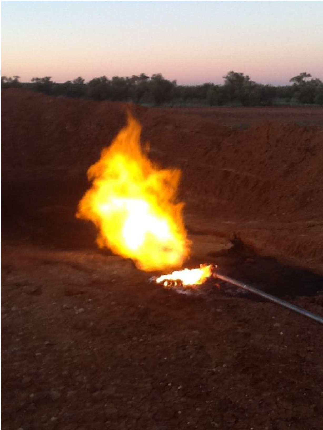
Flare from Tamarama- 1 testing the Patchawarra formation.
