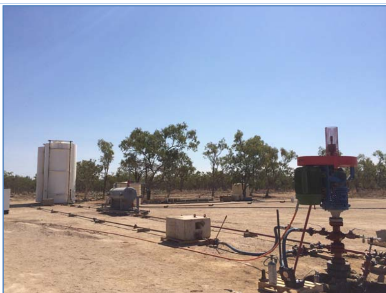
Figure 3: Egilabria 2 well - Well and flow test apparatus.
