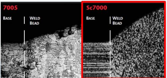
Significant grain refinement strengthens welds and eliminates hot cracks.
