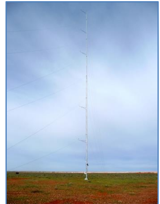
Wind monitoring mast, installed May 2014
