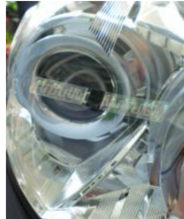
Figure 12: Tag with break on removal technology (BOR) adhered to a vehicle headlight
