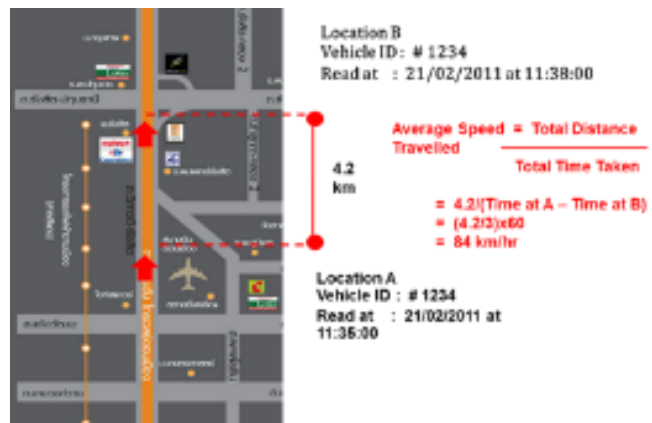
Figure 23: Method of calculating speed over a distance
