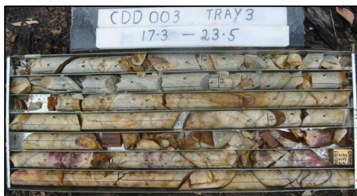
Figure 2. Supergene enriched copper zone in partially oxidised rock
