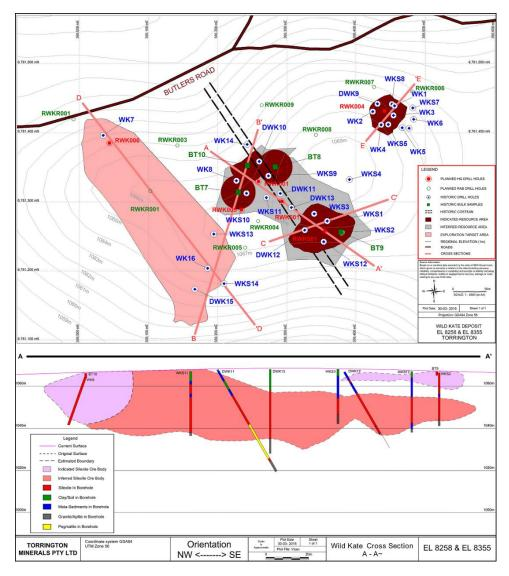
Figure 3: Wild Kate - Modelled Silexite Body and Resources showing simple ore geometry
