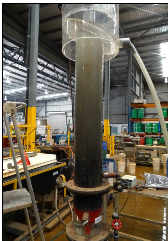
Elutriation Column with Hawsons material, Iron Ore Technical Centre, WA
