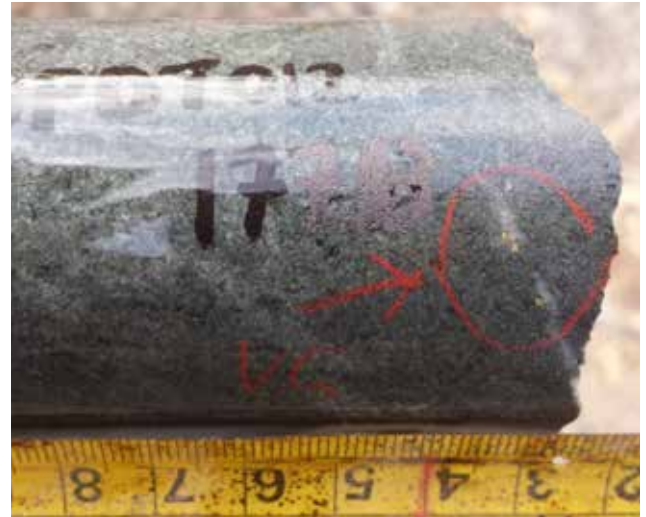
Figure 8 Visible gold logged within SPDT012 at 177.13m downhole. Diameter of NQ2 drill core is 50.5mm.
