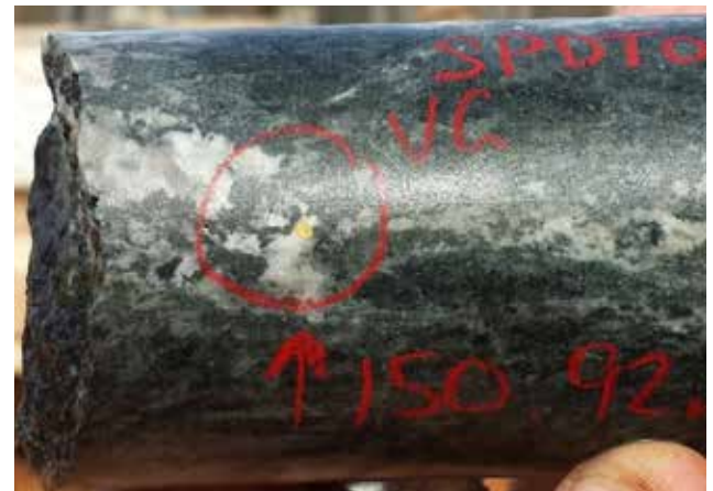
Figure 3 Visible gold logged within SPDT001 at 150.92m downhole. Diameter of NQ2 drill core is 50.5mm.
