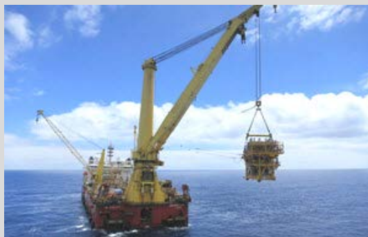
Sapura 3000 heavy lift vessel with Compressor Module suspended
