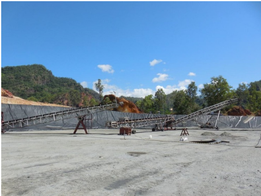
Image 4 : Gold Pit Leach Pad ready for stacking
