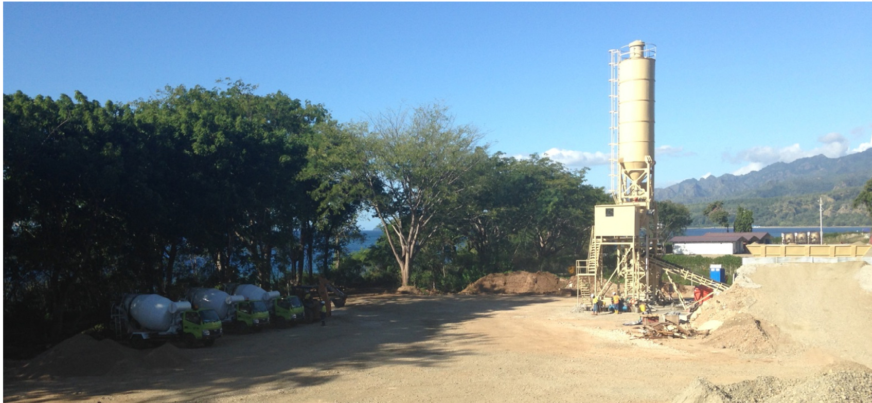
Concrete Batching Plant and Agitator Trucks
